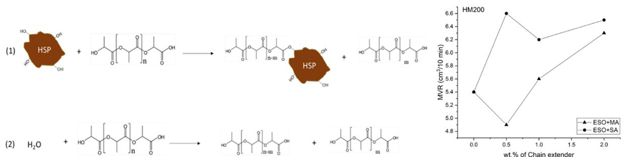
Figure 1. (a) Main reactions occurring during the preparation of PLA/HSP biocomposites, Reaction 1 involves a HSP solid particle; (b) Melt Volume Rate as a function of biobased chain extenders (ESO+MA and ESO+SA) percentage in PLA/PBSA based composite reinforced with HSP (HM200 type).
