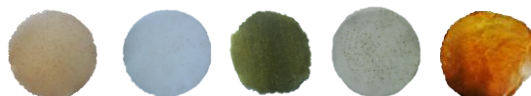
Figure 1. Composites films of biobased polymers and various waste materials produced by hot press moulding
